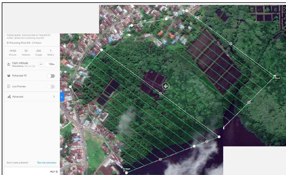
Figure 2. Flight plan for drone aerial mapping (figure generated using DroneDeploy).
