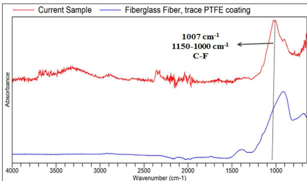
Figure 9. PTFE spectrum on the sample.
