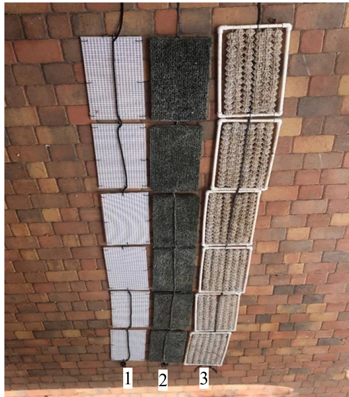
Figure 1. Displays the three different types of settlement collectors secured to polypropylene line: 1. egg crating; 2. door mat; 3. bioballs.
