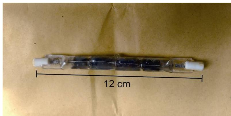
Figure 2. Halogen lamps.
