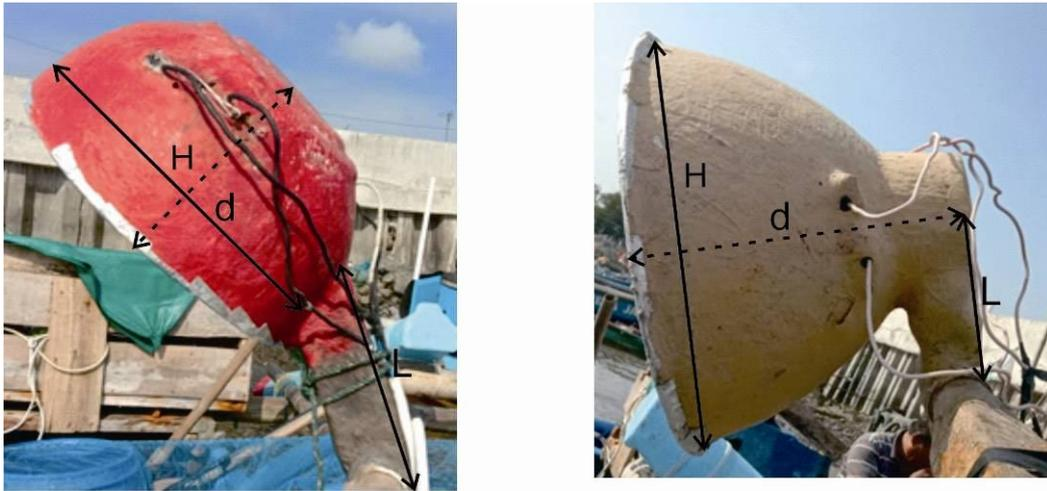
Figure 3. (left) Concave type reflector; (right) Conical type reflector (personal documentation, 2018).
