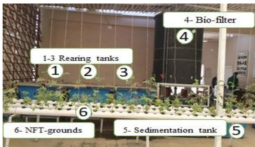
Figure 1. The design of the basic ASTAF-PRO aquaponic unit connecting RAS and hydroponic by a one-way valve (Osman et al 2021).
