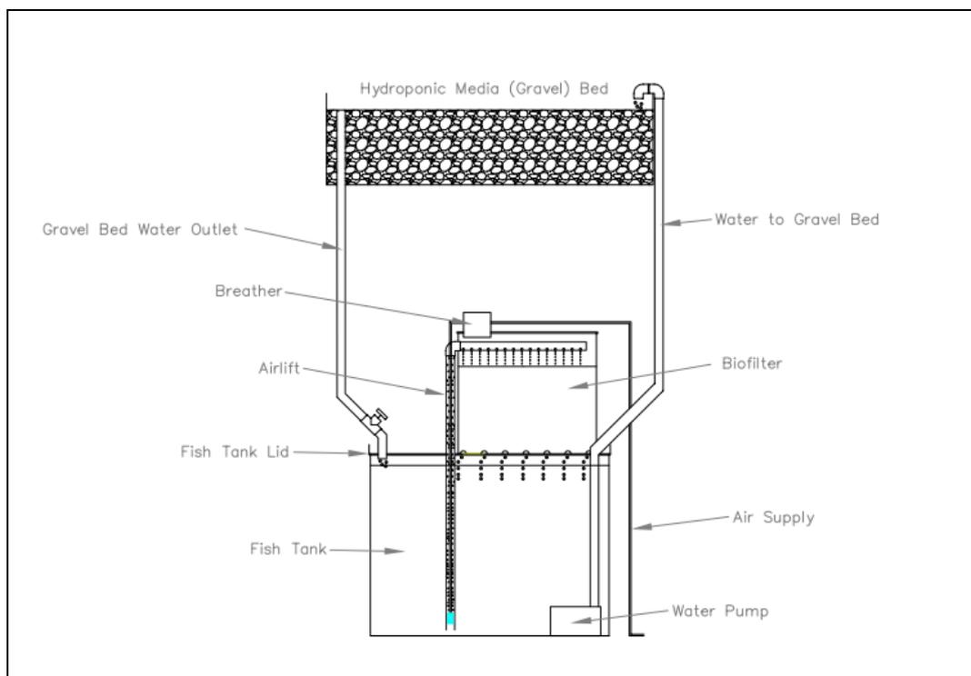
Figure 1. Schematic representation of a single, recirculating aquaponic test unit.
