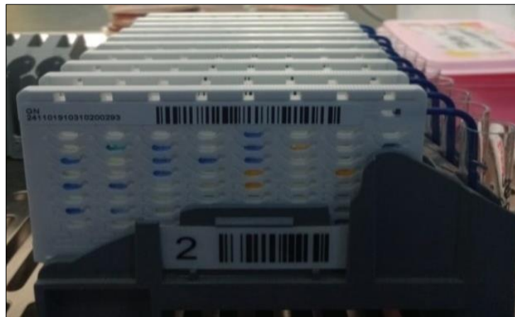
Figure 1. Identification card and disposable tube of Vitek-2 Compact along with the cassette (original).
