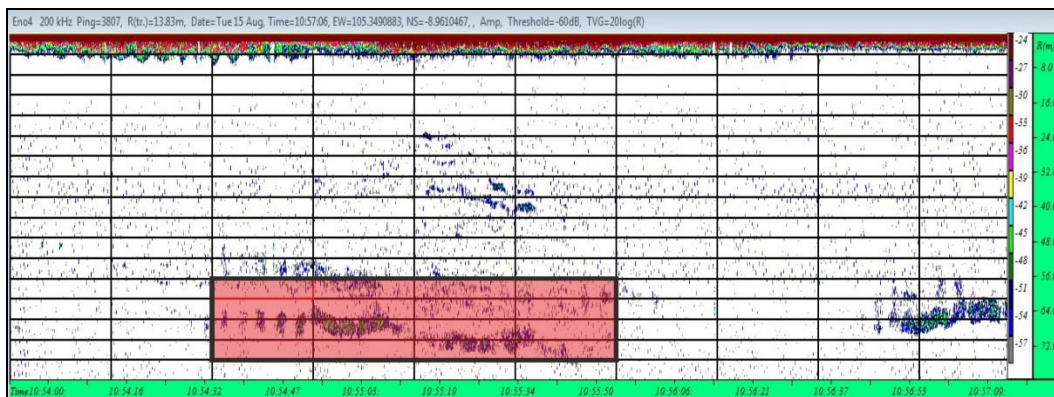
Figure 6. Echogram of fish movement during the day.
