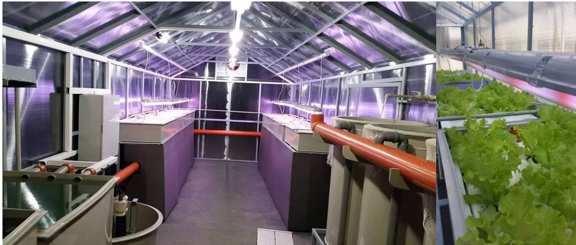
Figure 1. Aquaponic recirculation aquaculture system used in the current trial.
