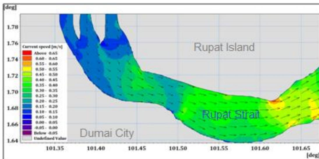
Figure 7. Hydrodynamic model at high tide.
