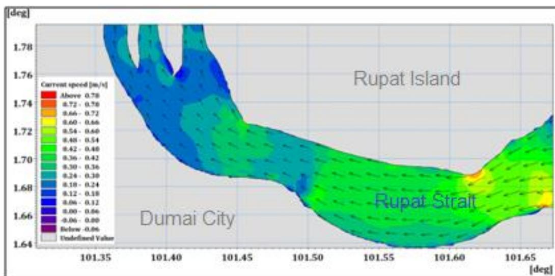
Figure 6. Hydrodynamic model at low tide.
