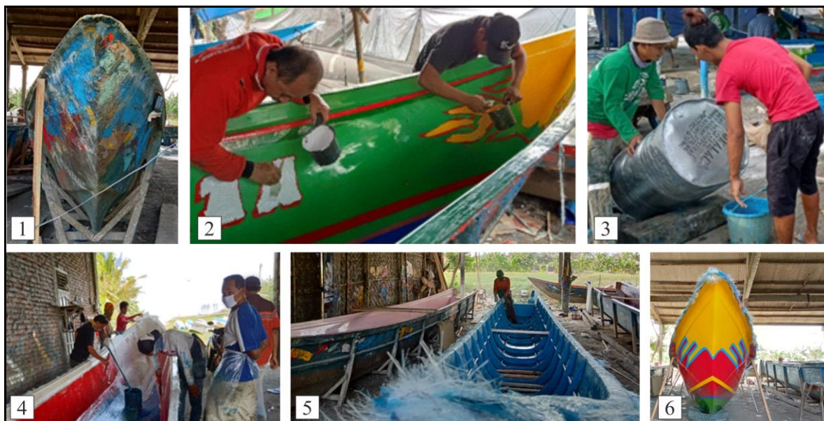
Figure 8. Process of production vessel. 1 - preparing the mould; 2 - drawing the ship's name, logo and style; 3 - preparation of laminated material; 4 - lamination process; 5 - installing the ship's frame and bulkhead; 6 - finishing.
