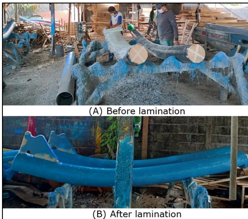
Figure 6. The process of forming the "katir" of a boat.
