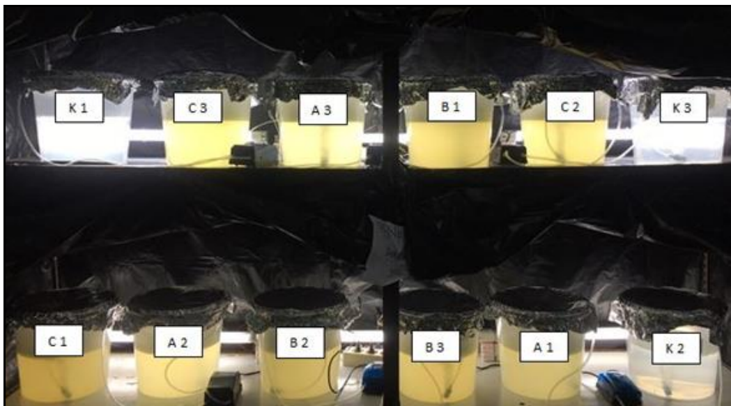
Figure 2. Culture setup of Chlorella pyrenoidosa . A - treatment with 10% tofu wastewater; B - treatment with 15% tofu wastewater; C - treatment with 20% tofu wastewater; K - control with 0% tofu wastewater; 1, 2, 3 - replications.
