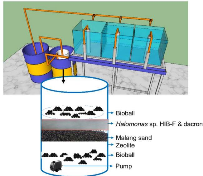
Figure 1. The design of the application system of *Halomonas* sp. HIB-F in a recirculation aquaculture system of *Litopenaeus vannamei* (Hastuti et al 2017; Hastuti et al 2019 modified).
