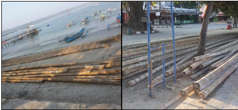
Figure 1. Bamboo Betung ( Dendrocalamus asper ) used to build a set lift net (original).
