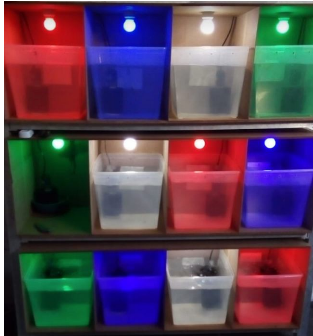
Figure 1. Photo of experimental setup (aquariums and filters) exposed to four colors LED lights (white, red, green and blue) during the experimental period. Tank in green space in middle row was removed for photo to show light barriers more clearly.
