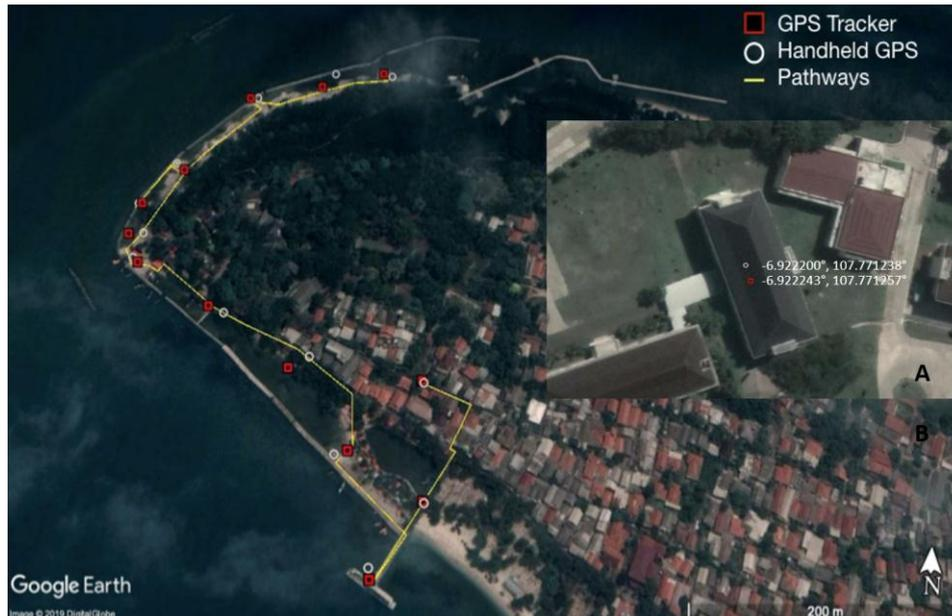
Figure 2. The testing positions between GPS tracker and GPS handheld Garmin A) 12 hours in the laboratory, B) field testing.
