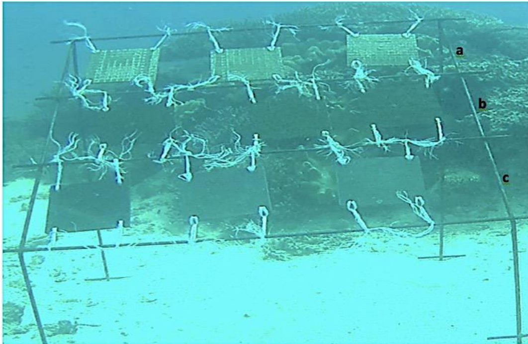
Figure 3. The placement of the collector substrates on the frame. (a) Ceramics; (b) Plate of mild iron drum; and (c) Andesite stone.
