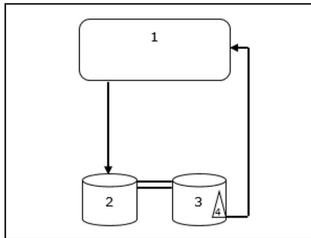
Figure 1. The layout scheme of the recirculating aquaculture system (1 - fish tank; 2 - physical filter; 3 - biological filter; 4 - pump).
