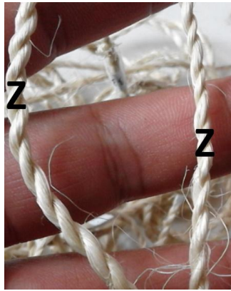
Figure 3. The direction of Z-twisted on ramie rope.
