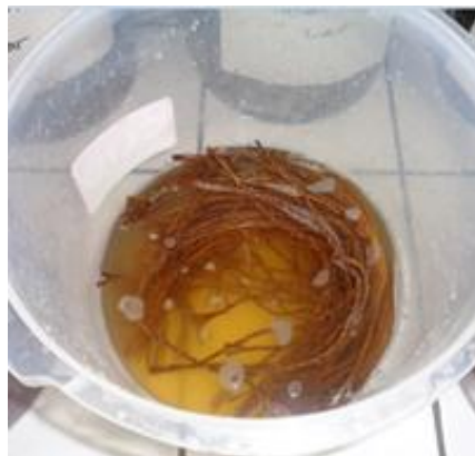
Figure 1. Immersion of ramie rope in 1% chitosan solution.
