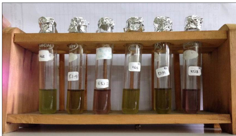
Figure 3. Antioxidant activity test on Dunaliella sp. using DPPH method.
